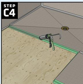
To install the straight extension piece(s) apply a 1/2" continuous bead of HYDRO-BLOK joint sealant along the shower pan notch, along the exposed foam edge of the shower pan, and along the corner extension notch. Apply a generous amount of joint sealant to the wallboard where the ends of the extension(s) will be located.
